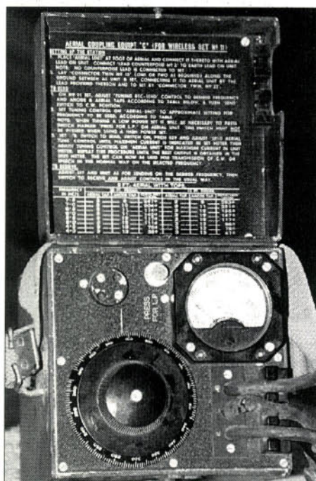
Fig. 2: The 'Aerial Coupling Equipment C' (For Wireless Set No. 11). This unit employs a variometer and is housed in a wooden case (see text).
